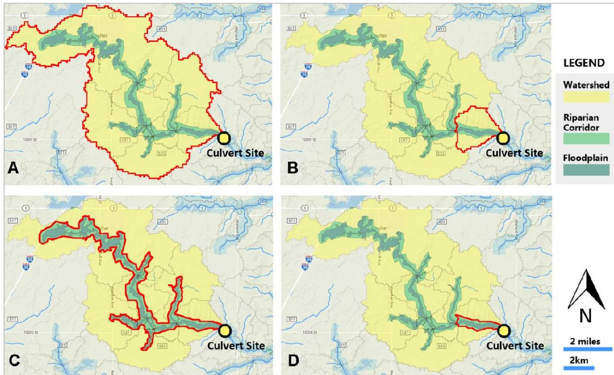
Fig. 2. Characterization of culvert upstream areas (highlight in red lines): (a) watershed, (b) local catchment, (c) riparian corridor (represented by the green buffer areas), and (d) immediate corridor upstream of culvert.
