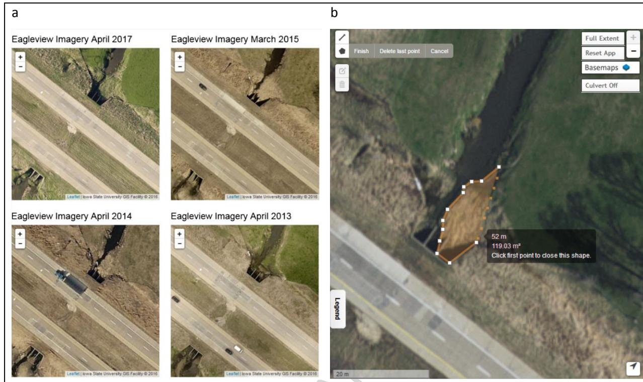
Fig. 3. The digital viewer for (a) displaying time-series aerial imagery in the culverts' vicinity and (b) delineating the area of sediment depositions at a culvert.
