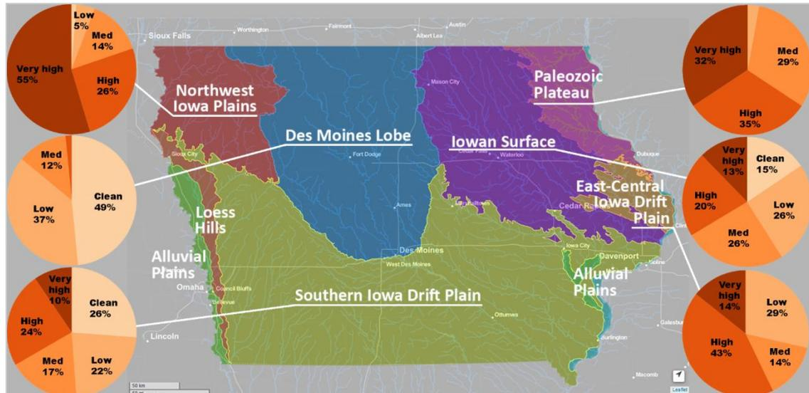
Fig. 7. Spatial variation of the culvert sedimentation degrees across different landform regions in Iowa.
